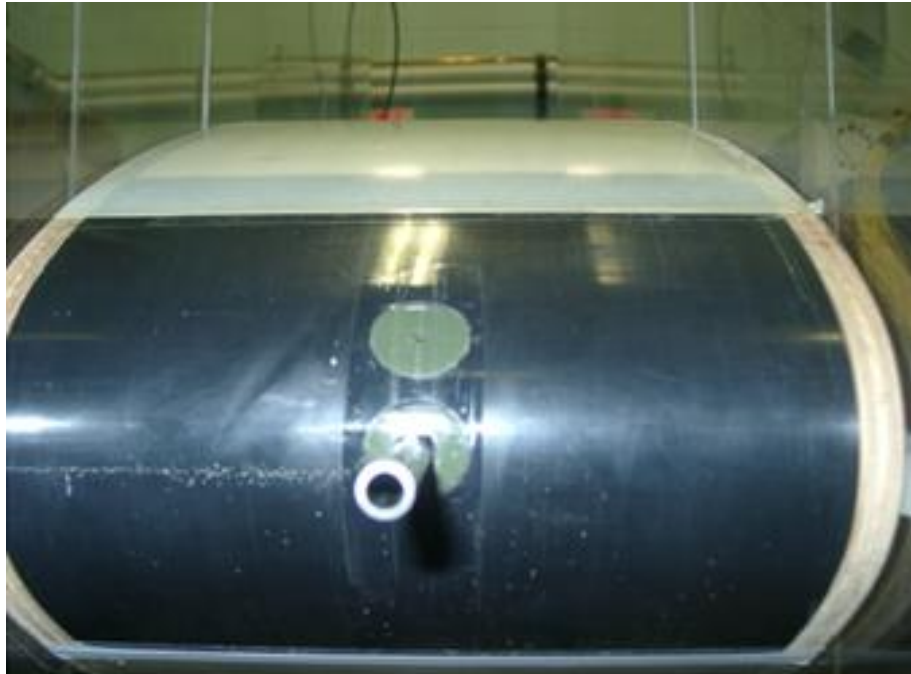
Figure 31. Front view of the 0.1016 meter cylindrical leading edge vane.
