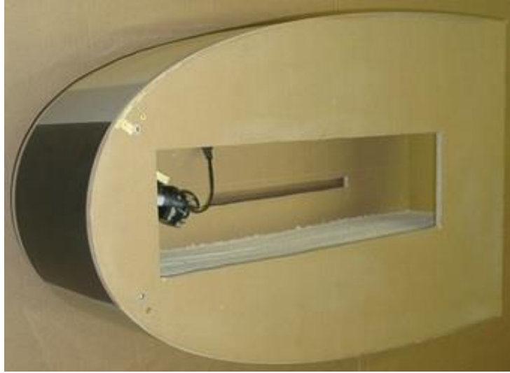
Figure 6. The 0.4064 meter cylindrical leading edge vane.
