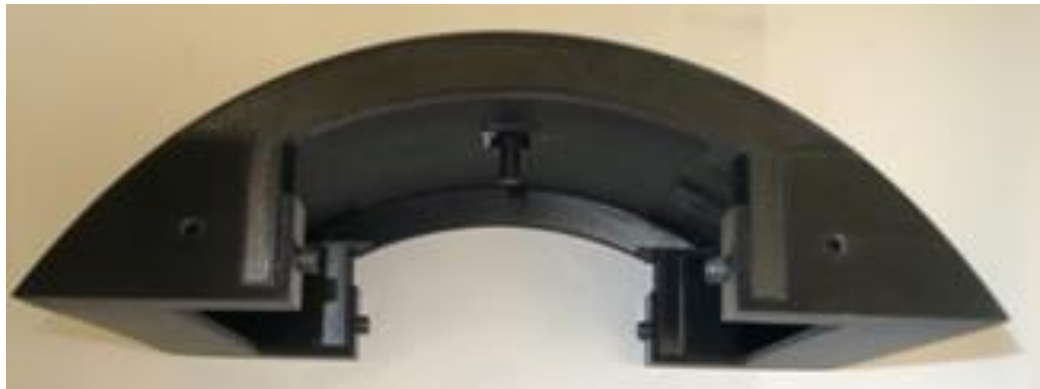
Figure 7. The assembled 0.4064 meter cylindrical leading edge tip.
