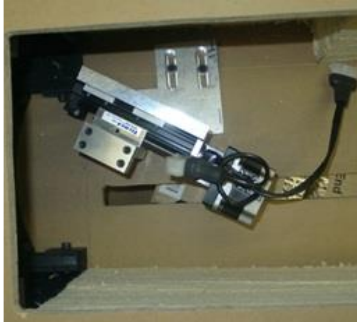
Figure 15. Traversing equipment mounted in test apparatus.
